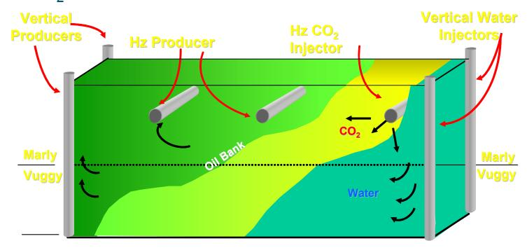
CO<sub>2</sub> is injected at high pressure where it essentially acts as a solvent for oil:
