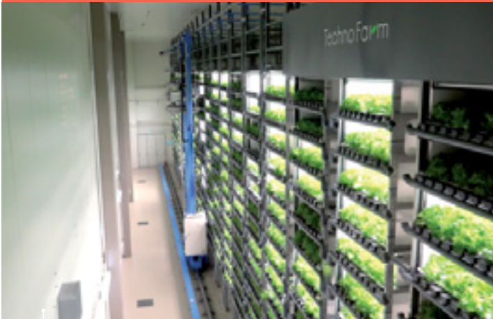
Automated vertical farm Techno Farm Keihanna, capable of producing 30,000 heads of lettuce per day in Kyoto, Japan - ©Spread
